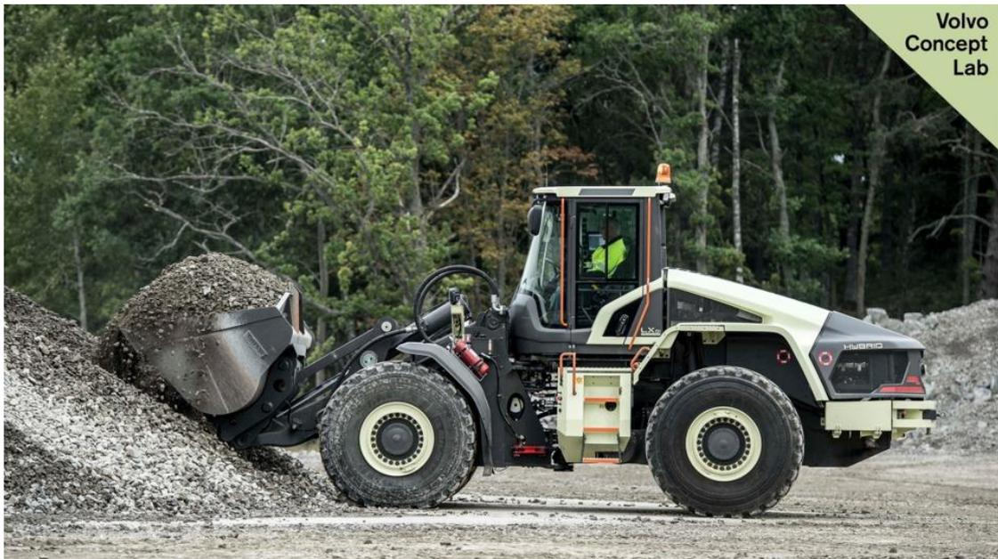
The LX1 wheel loader from Volvo Construction Equipment (Volvo CE) is a series hybrid that incorporates a driveline consisting of electric drive motors mounted at the wheels, electric driven hydraulics, a battery energy storage system, a significantly smaller diesel engine and new machine architecture. It's this combination that enables the substantial gain in fuel efficiency. Tests at the Redwood Landfill and Recycling Center in California show an average improvement of 50% in fuel efficiency.
