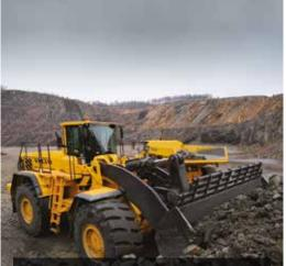
**One L350F wheeled loader** loading 800 tonnes/hour would produce over 5 million tonnes/year.
