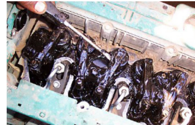
Engine full of dirt and oil sludge
