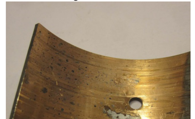
Worn main bearing
