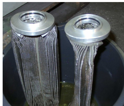
Collapsed non-genuine filters
