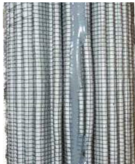
Bad joints on low quality filters
