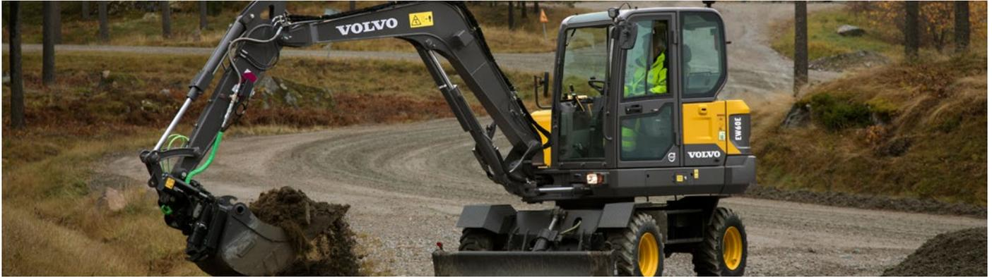
**3. You'll save on labor and cleanup** — With top speeds of approximately 20 mph, you can avoid having to use a lowboy and a CDL for around-town work. Outfit the trailer with overrun brakes, and you can haul up to an 8.5-ton trailer with all your supporting tools and attachments. That saves time and labor. Wheeled excavators don't damage asphalt like tracked machines do, which means less time and money spent on cleanup.
