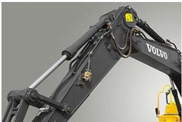
Excavator boom and arm
