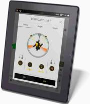
Prevents the swing exceeding pre-set limits, to avoid contact with side obstacles. Cannot be overridden with the joystick.
