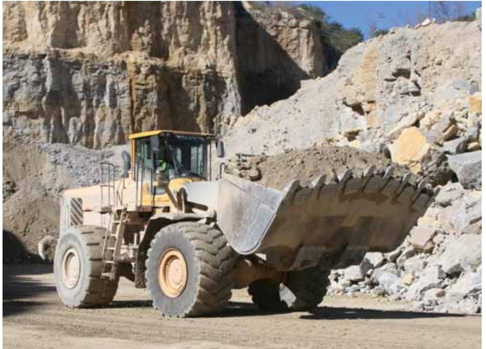
The Volvo L350F works a one-quarter-mile load-and-carry operation at Nimtz Quarry.
