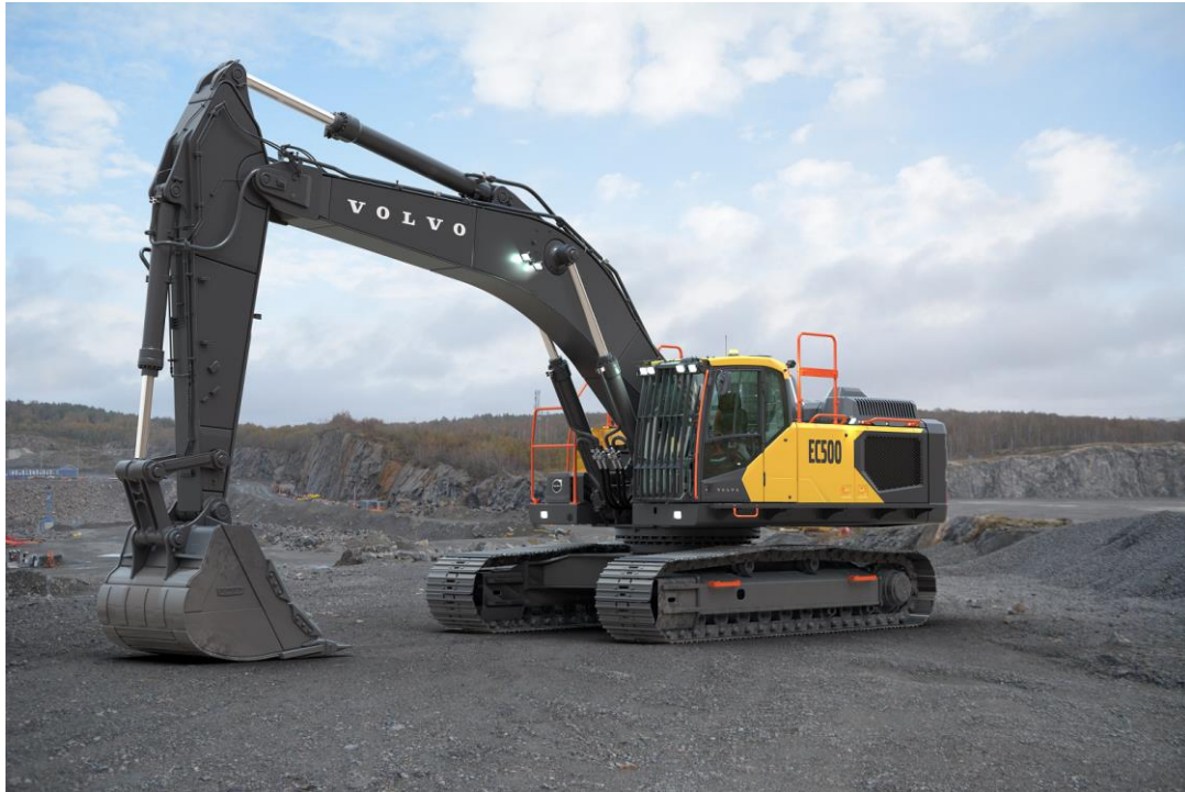
The EC500 excavator is fitted with Volvo Smart View with Obstacle Detection
