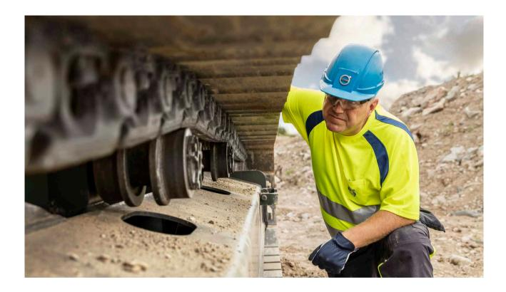
A poorly maintained undercarriage affects machine safety, reduces productivity, and can damage other vital components.
