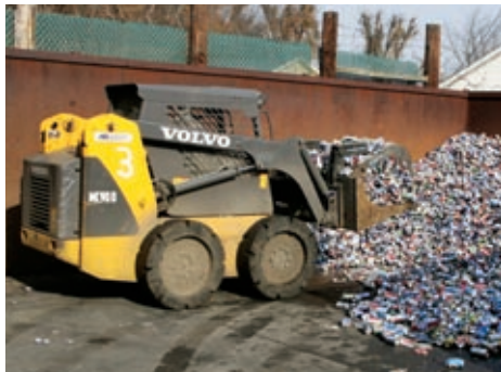
A Volvo MC90B picks up aluminum cans to deliver to the baling machine.
