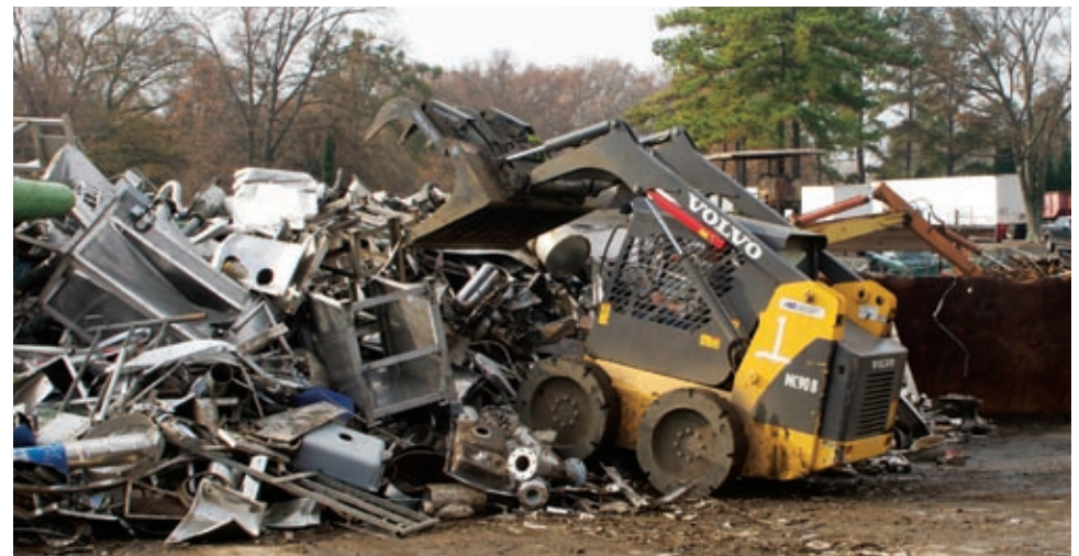
A Volvo MC90B skid steer loader works the stainless steel metal stockpile.
