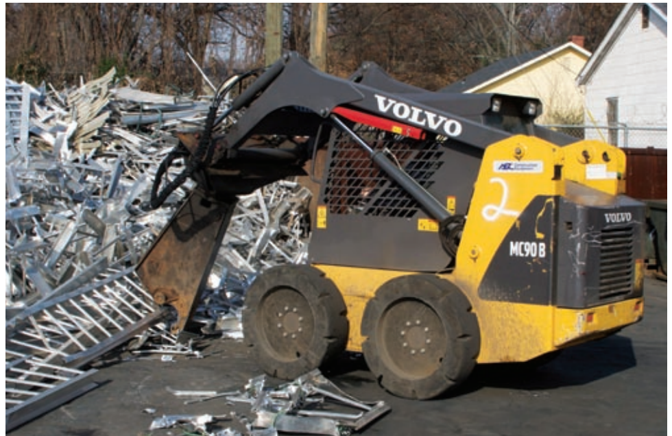
One of Mintz' Volvo MC90B skid steer loaders is fitted with a shear, shown here cutting up scrap aluminum.
