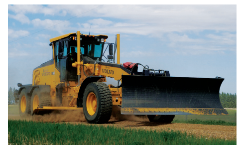
The Volvo G940 in action. Certain road conditions require the blade cutting edge to be changed twice a day.
