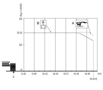
A Maximum tipping capacity B Rated capacity
