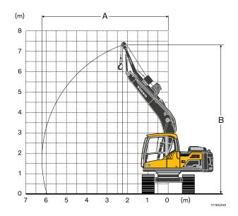
Boom + Rotating pipelayer kit = 5.98 m A Maximum working reach: 6205 mm B Maximum working height: 7317 mm
