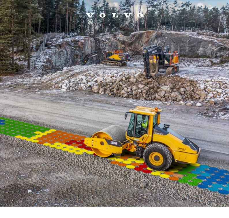
Intelligent Compaction for Volvo Soil Compactors
