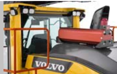
Fire suppression system
