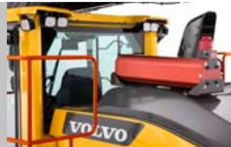
Fire suppression system
