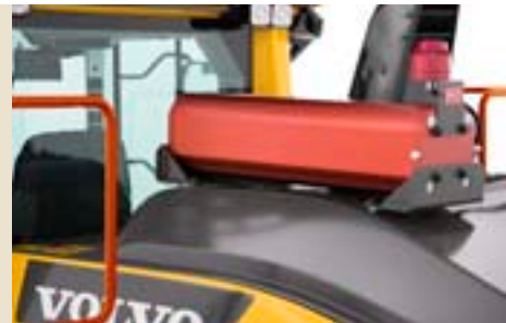
Fire suppression system
