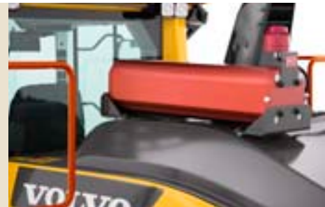
Fire suppression system
