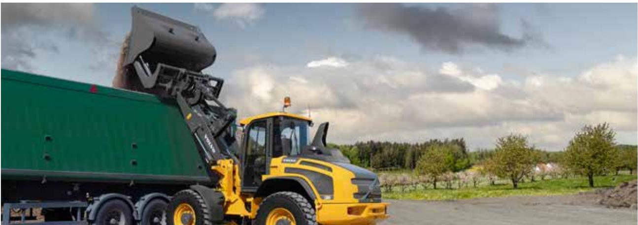
The bucket comes with a pre-drilled cutting edge made from Hardox 400 steel. It can be equipped with a 1 or 3-piece bolt-on edge made from Hardox 400 as an option. Wear parts can be found on page 24.
