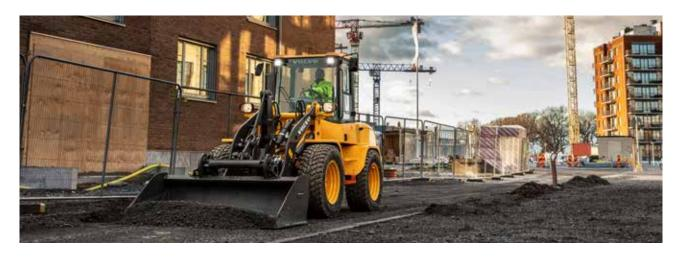
The bucket comes with a pre-drilled cutting edge made from Hardox 400 steel. It can be equipped with a 1 or 3-piece bolt-on edge made from Hardox 400 as an option. Wear parts can be found on page 24.
