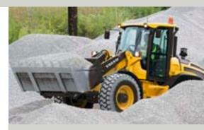
• 100% operator selectable differential locks provide maximum traction.
