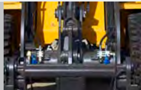
3 rd and 4 th hydraulic circuit
