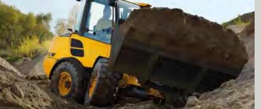
The articulating/oscillating joint keeps it stable.
