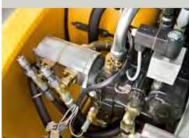
Separate working and steering hydraulic pumps.
