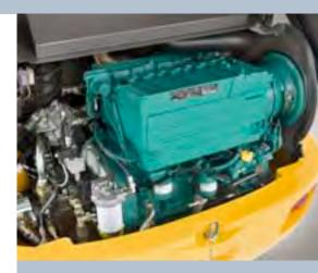
· High-performance, 4-cylinder Volvo diesel engine.
