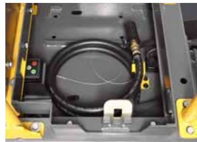
Fuel fill pump
