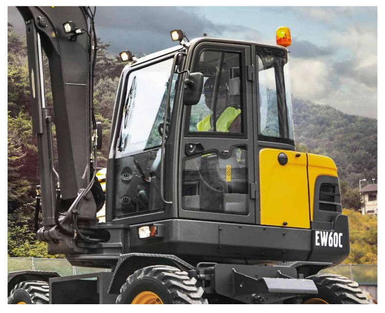
The Volvo Care Cab has excellent all-around visibility with a very large, glazed surface area on all four sides, high-capacity climate control and adjustable steering column. The responsive controls allow the operator to set the work speed without leaving the seat.
