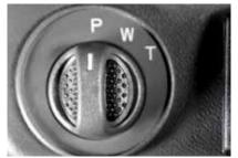
for all work conditions. Rotary type work mode control switch is convenient for both work and travel.
