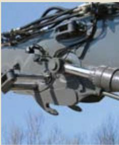
Innovative **hydraulic modular joint** uses a **hydraulic lock** mechanism to release digging equipment and **change from high reach** demolition boom to a standard backhoe configuration in **less than 30 minutes**. The feature greatly enhances versatility.
