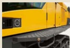
**Punched plate** is welded to the top of the rail along the cab entrance to provide sure grip for the operator.
