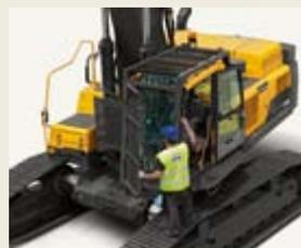
**Frame-mounted FOG protects the operator**
