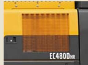
**Double-thickness side doors** on both sides of the superstructure protect coolers and pumps in the event of a side impact, and enhance overall machine life.
