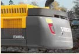
**Hydraulic Removable Counter weight option** Removable counterweights are easier to remove and install using Volvo's hydraulic cylinder and linkage system.
