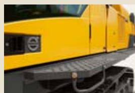
**Punched plate** is welded to the top of the rail along the cab entrance to provide sure grip for the operator.
