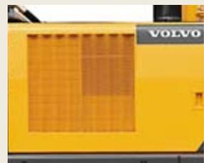
**Micro mesh screens keep particles from coolers**
