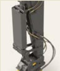
**Bucket and boom cylinder guards** protect rods, cylinders, HRVs and piping from falling objects. These steel jackets reduce the chance of machine damage and improve uptime on all types of demolition jobs.
