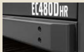
The bolt-on **side impact protection system** protects the superstructure from damage.
