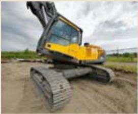
**Tilting cab pivots up to 30 degrees** for enhanced visibility and reduced fatigue on high-reach jobs. Standard on Ultra High Reach (HR) models and optional on Standard Demolition Excavator models.
