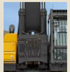
**Boom Cylinder Protection System** visible through the plate from the cabin for visibility to the right track.
