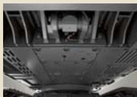
Enhanced 8 mm (0.32 in) **under-guarding of the superstructure** and 10 mm (0.39 in) **guarding under the slewing ring**, with bolt-head protection.
