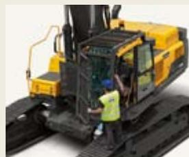
**Frame-mounted FOG protects the operator**
