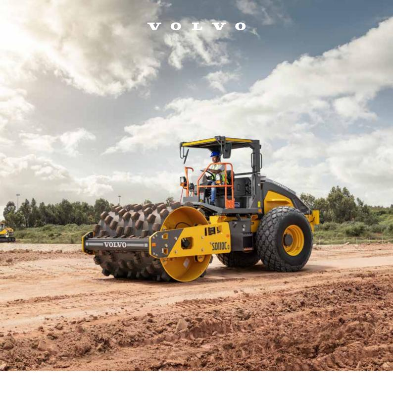
Volvo Single Drum Compactors 11.1 t 74 kW
