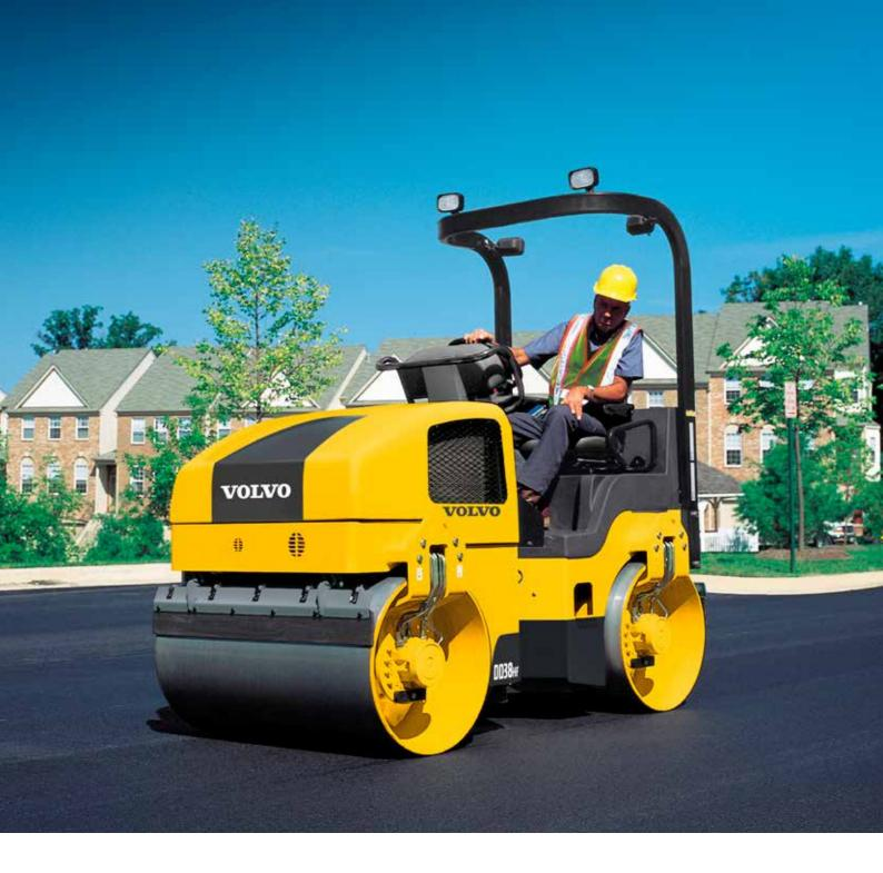
Volvo Double Drum Compactors 3.8 t / 8,400 lb 31.3 kW 42 hp
