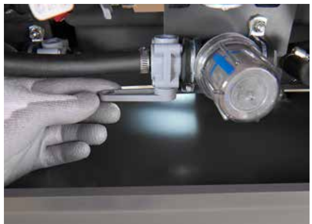
Quick drain freeze prevention
