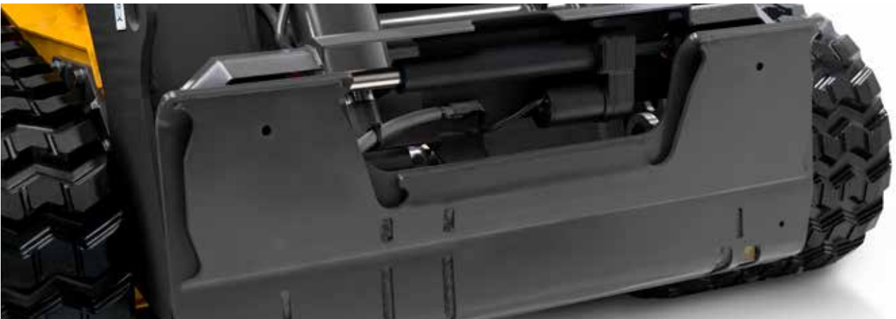
Volvo assisted attachment bracket allows the operator to change attachment from the seat
