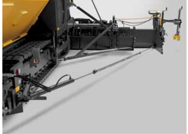
Hydraulic height Adjustment of Extendable Screed
