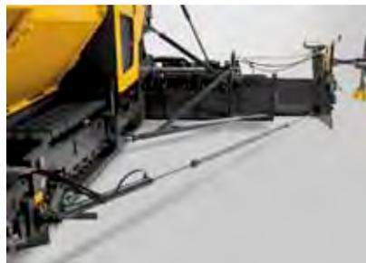
**Hydraulic auger height adjustment**
