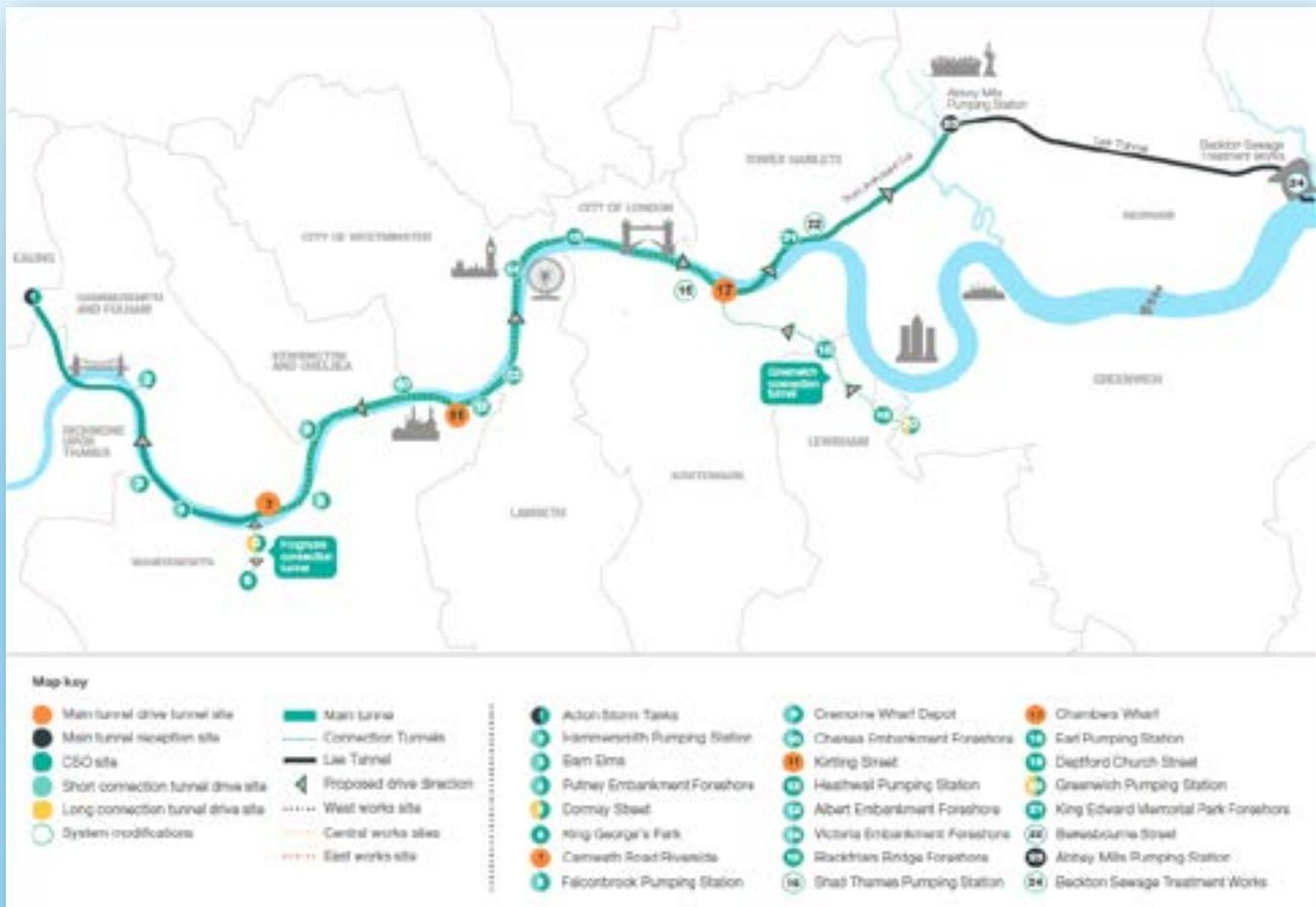
The Thames Tideway project is building a 25km tunnel or 'super sewer' underneath the Thames to help with pollution due to overflowing with high rainfall levels.
