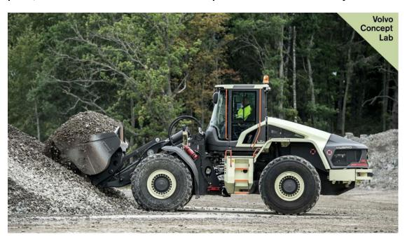
The LX1 wheel loader from Volvo Construction Equipment (Volvo CE) is a series hybrid that incorporates a driveline consisting of electric drive motors mounted at the wheels, electric driven hydraulics, a battery energy storage system, a significantly smaller diesel engine and new machine architecture. It's this combination that enables the substantial gain in fuel efficiency. Tests at the Redwood Landfill and Recycling Center in California show an average improvement of 50% in fuel efficiency.
