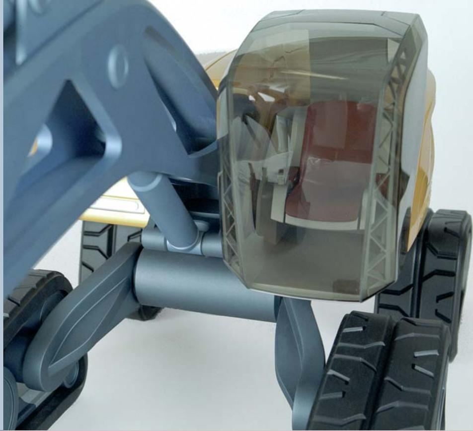
*The engine acts as the machine counter weight, which moves all the time to compensate for the forces on the boom.*
