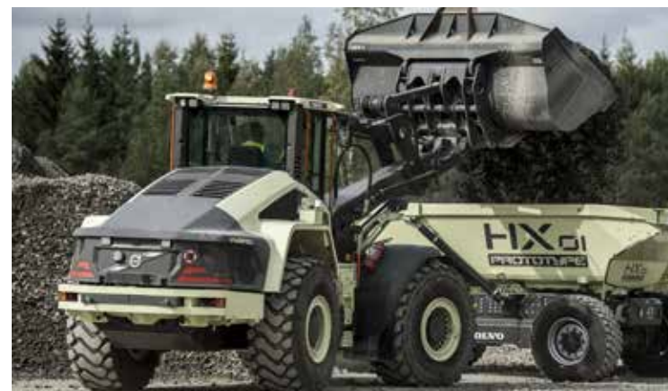
Concept HX1 autonomous, battery-electric load carrier and LX1 prototype electric hybrid wheel loader unveiled at Xploration Forum, Eskilstuna, Sweden
