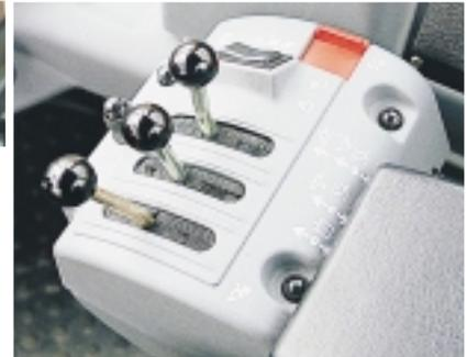
Pilot operated fingertip hydraulic levers provide easy control of the hydraulic functions. The adjustable hydraulic lever console also features a rocker switch for forward/reverse shifting and a 1<sup>st</sup> gear kickdown button.
