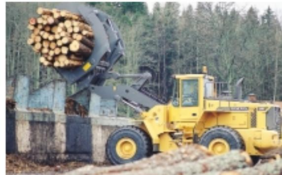
TP linkage comes into its own in timber applications. No other system provides such high breakout torque throughout the lift cycle.
