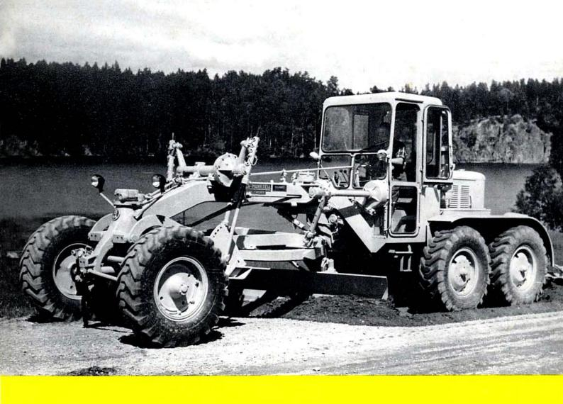
The Bolinder-Munktell VHK 100 is a grader built for hard work on all kinds of jobs. Every component has been designed to take the heaviest stresses. Correct weight distribution allows full use of the lugging capacity of the powerful diesel engine, so that the VHK 100 has the pull you need on heavy construction projects.
