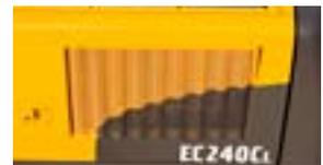
**Engine air-intake screen** prevents larger particles from entering the radiator compartment and maintains cooling performance for uptime and reliability.
