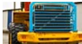
**Radiator grille guard** protects grille, cooling fan, radiator and condenser cores from damage. It is hinged to facilitate easy cleaning and maintenance.
