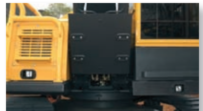
Boom cylinder guard. Optional boom foot riser increases boom and arm reach and overall machine stability.
