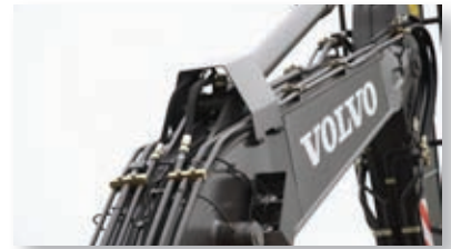
Boom and arm with HD forestry guarding, integrated piping, hydraulic cylinder and work light guarding.
