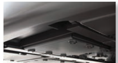
Enhanced 8 mm underbody guarding with bolt-head protection keeps forestry debris and rocks from damaging the super structure.
