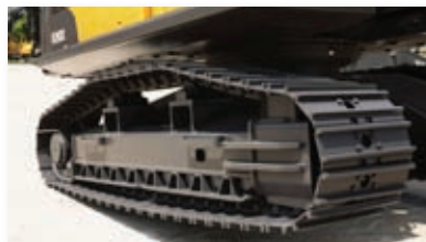
HD full length track rock guards. Dual mounted bottom rollers on top. Reinforced idlers with derail guards.
