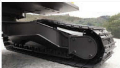
Purpose-built, high-walker undercarriage and high capacity track motors with HD track motor covers.
