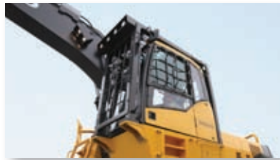
Volvo Forestry Care Cab with standard 457 mm cab riser and full forestry guarding meets global safety standards.
