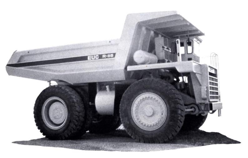
Safe, efficient and comfortable are the key words for the Euclid cab. It is offset to the left and positioned well forward for maximum operator visibility. Glass area totals 2.11 m² (22.7 ft²). Operator controls and instrumentation are simple and within easy reach. Thick foam insulation, tinted safety glass and an adjustable driver's seat combined to form a comfortable operator environment.
