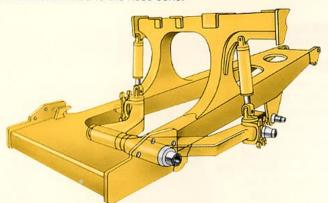
NEOCON struts outperform competitive strut designs by improving isolation, stability, and control. Improved isolation means reduced impact loading on the structural members of the machine and greater operator comfort, resulting in longer equipment life and increased productivity. Improved stability means more consistent dynamic response of the machine to fluctuating load energy, resulting in predictable machine performance. And improved control means better machine maneuverability.
