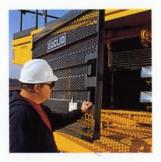
The swing-out front grille provides easy access to the radiator, lights, air conditioner condenser and brake accumulators.
