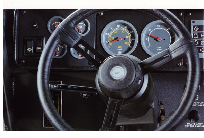
A wrap-around style dashboard positions controls within easy reach of the operator and allows good visual contact with all instrumentation.
