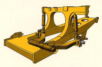
NEOCON struts outperform competitive strut designs by improving isolation, stability, and control. Improved isolation means reduced impact loading on the structural members of the machine and greater operator comfort, resulting in longer equipment life and increased productivity. Improved stability means more consistent dynamic response of the machine to fluctuating load energy, resulting in predictable machine performance. And improved control means better machine manueverability.
