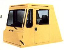
structurally sound cab. Foam rubber lining material along with foam rubber-backed carpeting and multiple layered floor mat act to absorb sound and control interior temperature. A properly maintained cab from VME, tested with doors and windows closed per work cycle procedures in ANSI/SAE J1166 (1990), results in an operator sound exposure Leq (Equivalent Sound Level) of 79dB(A). A three-point rubber iso-mount arrangement to the deck surface minimizes vibration to the operator compartment.
