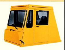
a more structurally sound cab. Foam rubber lining material along with foam rubber-backed carpeting and multiple layered floor mat act to absorb sound and control interior temperature. A properly maintained cab from Euclid, tested with doors and windows closed per work cycle procedures in SAE J1166 (1990), results in an operator sound exposure Leq (Equivalent Sound Level) of 79 dB(A). A three-point rubber iso-mount arrangement to the deck surface minimizes vibration to the operator compartment.
