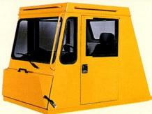
sound cab. Foam rubber lining material along with foam rubber-backed carpeting and multiple layered floor mat act to absorb sound and control interior temperature. A properly maintained cab from Euclid, tested with doors and windows closed per work cycle procedures in SAE J1166 (1990), results in an operator sound exposure Leq (Equivalent Sound Level) of 79 dB(A). A three-point rubber iso-mount arrangement to the deck surface minimizes vibration to the operator compartment.
