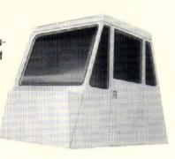
layered floor mat act to absorb sound and control interior temperature. A three-point rubber iso-mount arrangement to the deck surface minimizes vibration to the operator's compartment.
