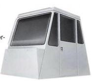
Unparalleled Operator Comfort and Convenience for Increased Productivity. This ergonomically designed cab includes the Isringhausen six-way adjustable air seat, tilt steering wheel, in-dash duct work for filtered ventilation, and a tumblehome acoustical design for reduced interior sound levels which rival those found in better automobiles. The seat back on the fully upholstered trainer's seat folds down to serve as a tray at break time.
