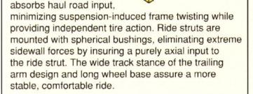
The suspension struts employ gas and Neocon-x fluid as the energy-absorbing media. This suspension continues to absorb energy when extreme dynamic loads are generated which significantly contributes to improved isolation of the operator and machine components.
