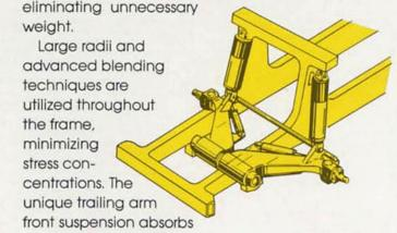
haul road input, minimizing suspension-induced frame twisting while providing independent tire action. Ride struts are mounted with spherical bushings, eliminating extreme sidewall forces by insuring a purely axial input to the ride strut. The wide track stance of the trailing arm design assures a more stable, comfortable ride.
